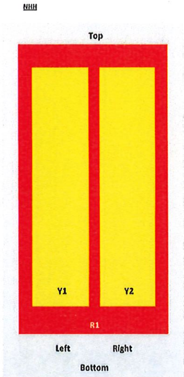
View from the front of the antenna (Sizes of colored boxes are not true depictions of array sizes)
